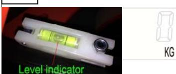
The forks are at the reference height (about 15.5CM) , and the Level indicator is in the middle of Level. Check the zero value in the display.
