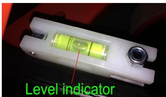
When the Level Indicator will be horizontal, lift the pallet truck slowly till the level indicator in the middle of the level.
