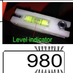
Pick up a load and lift it to the reference height, the Level Indicator is in the middle of Level at
