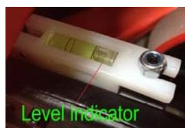
When the load has been lifted too high, the level indicator will not be in the middle of the level.
