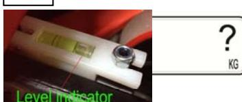
Lift the forks to the reference height and check the zero value in the display
