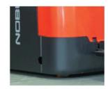
The use of apron with 8 mm thickness allows to ensure the robustness of chassis and its strength even in case of collision against objects. The strong battery cover made out of steel helps to provide a high level of strength for this part.
