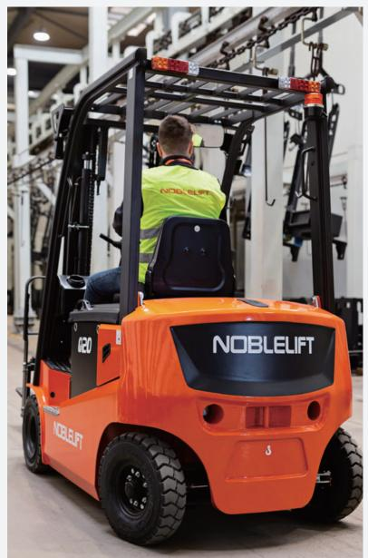
The trucks are equipped with **Curtis** controllers, **CAN-bus** technology makes the diagnostic and troubleshooting easier. The use of proved and certified components helps to
