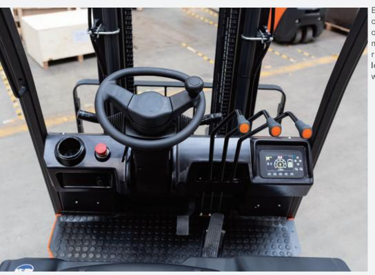
Ergonomic hydraulic controls for comfort operation with wide mast view and easy right-sided control levers and steering wheel with knob.
